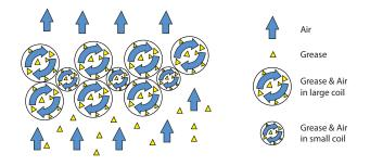
1. Air and Grease go into the Veritech filter
